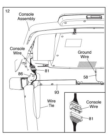
Set the console assembly on the brackets on the Handrails (86). Make sure not to pinch any wires. Insert the excess Upright Wire (81) into the Right Upright (90).
