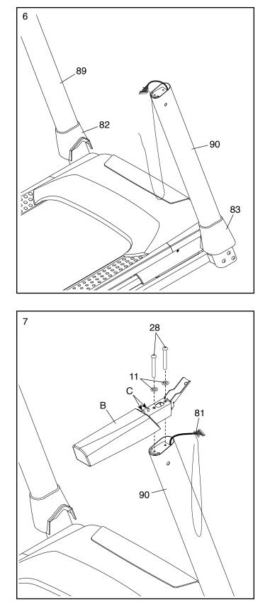
7. Identify the right handrail assembly (B).
