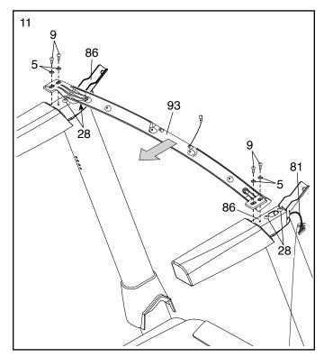
12. With the help of a second person, hold the console assembly near the Handrails (86) (only one side is shown).
