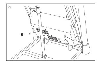
Lower the treadmill. Next, remove the indicated #8 x 3/4" Screws (6). Carefully slide the Motor Hood (57) off.
