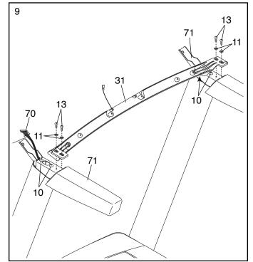
10. With the help of a second person, hold the console assembly near the left Handrail (71) and the right Handrail (not shown).
