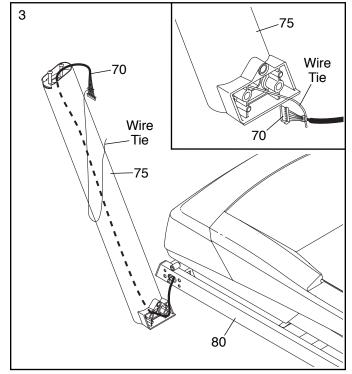
4. Hold the Left Upright (75) against the Base (80). Be careful not to pinch the wires. Partially tighten three 3/8" x 4" Screws (4) with three 3/8" Star Washers (5) into the Left Upright and the Base. Do not fully tighten the Screws yet.
