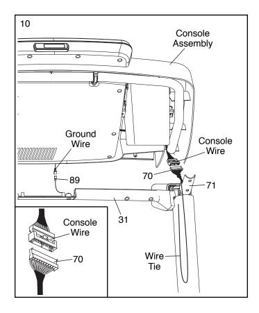
11. Set the console assembly on the left and right Handrails (71). **Make sure that no wires are pinched.** Insert the excess Upright Wire (70) behind the Console Frame (87).
