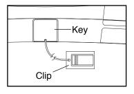
a moment, the displays will light. IMPORTANT: In an emergency, the key can be pulled from the console, causing the walking belt to slow to a stop. Test the clip by carefully taking a few steps backward; if the key is not pulled from the console, adjust the position of the clip.
