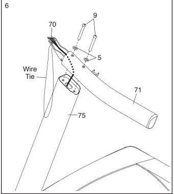
Attach the Right Handrail (72) to the Right Upright (76) with two 3/8" x 3 1/2" Screws (9) and two 3/8" Star Washers (5). Start both Screws, but do not tighten them yet.
