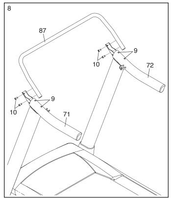
9. With the help of a second person, hold the console assembly near the Left Handrail (71) and the Right Handrail (not shown).
