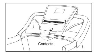
To measure your heart rate, **stand on the foot rails** and hold the pulse bar with your palms on the metal contacts for approximately ten seconds; **avoid moving your hands.** When your pulse is detected, a heart symbol in the calorie display will flash each time your heart beats, one or two dashes will appear, and then your heart rate will be shown. For the most accurate heart rate reading, continue to hold the contacts for about 15 seconds.
