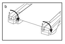
Using the hex key, turn both idler roller screws clockwise, 1/4 of a turn. When the walking belt is correctly tightened, you should be able to lift each edge of the walking belt 2 to 3 in. (5 to 7 cm) off the walking platform. Be careful to keep the walking belt centered. Then, plug in the power cord, insert the key, and carefully walk on the treadmill for a few minutes. Repeat until the walking belt is properly tightened.
