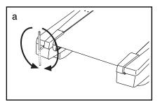
ing belt has shifted to the left, use the hex key to turn the left idler roller screw clockwise 1/2 of a turn; if the walking belt has shifted to the right, turn the left idler roller screw counterclockwise 1/2 of a turn. Be careful not to overtighten the walking belt. Then, plug in the power cord, insert the key, and run the treadmill for a few minutes. Repeat until the walking belt is centered.
