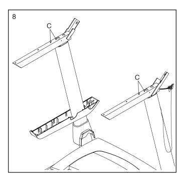
Set the console assembly face down on a soft surface to avoid scratching the console assembly. Remove and save the four 5/16" x 1/2" Screws (4). They will be used in the next step.
