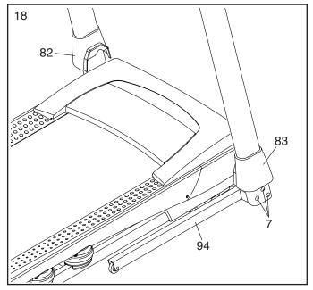
19. Make sure that all parts are properly tightened before you use the treadmill. If there are sheets of plastic on the treadmill decals, remove the plastic. To protect the floor or carpet, place a mat under the treadmill. To avoid damage to the console, keep the treadmill out of direct sunlight. Keep the included hex keys in a secure place; one of the hex keys is used to adjust the walking belt (see pages 30 and 31). Note: Extra parts may be included.
