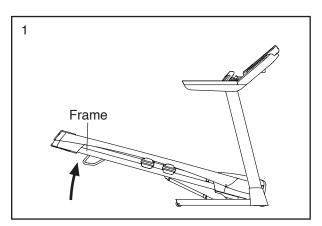
2. Raise the frame until the storage latch locks in the storage position. **CAUTION: Make sure that the storage latch locks.**
