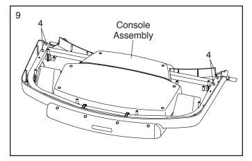
10. Set the console assembly on the Left and Right Handrails (86, 87). Make sure not to pinch any wires (D, 81).
