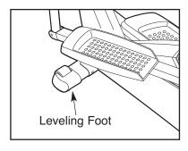
during use, turn one or both of the leveling feet under the front stabilizer until the rocking motion is eliminated.
