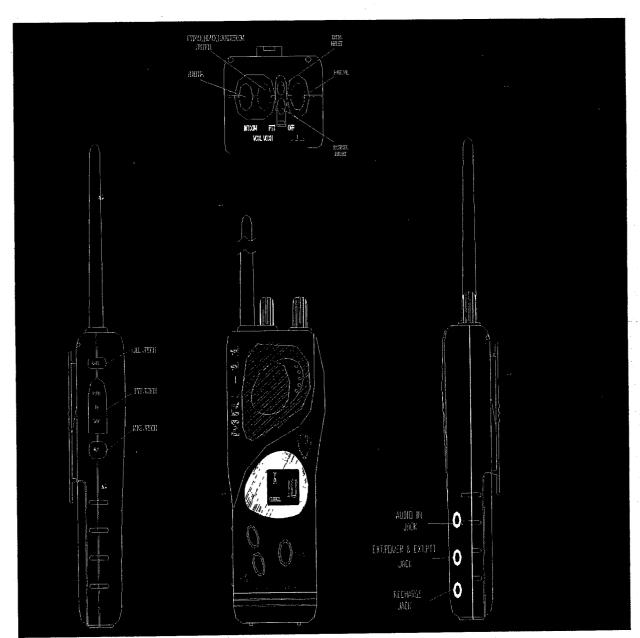
NOTE: The antenna is permanently attached to the radio. Do not attempt to remove.
