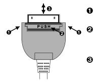
Support the sides of the connector with your thumb and forefinger of one hand.
