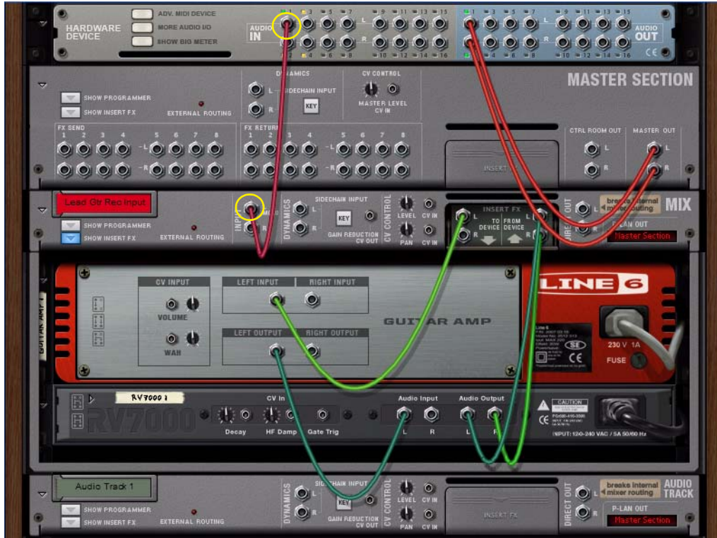
Direct routing of an Input signal from the Reason Hardware Device to the Mix Channel device
