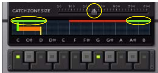
The Catch Zones for the selected notes C and G in a custom scale, with the C note Catch Zone “wrapped around” to cover also notes B and A#.
