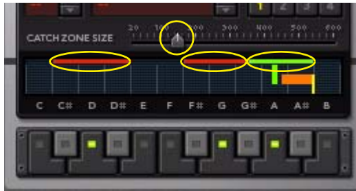
The Catch Zones for the selected notes D, G and A in a custom scale.
