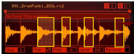
Slices 3, 5, 8 and 11 selected for playback in Slice Trig mode, forcing them to play back alternating
