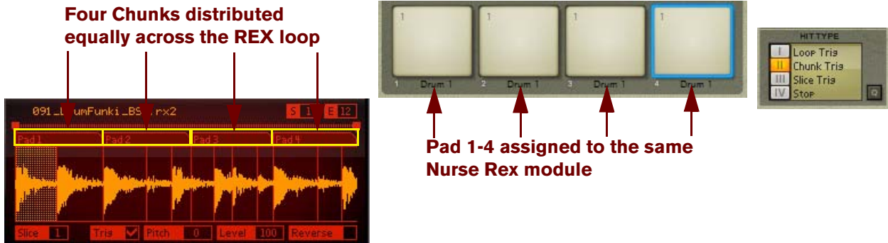
Four pads assigned to the same REX loop and Hit Type set to “Chunk Trig”
