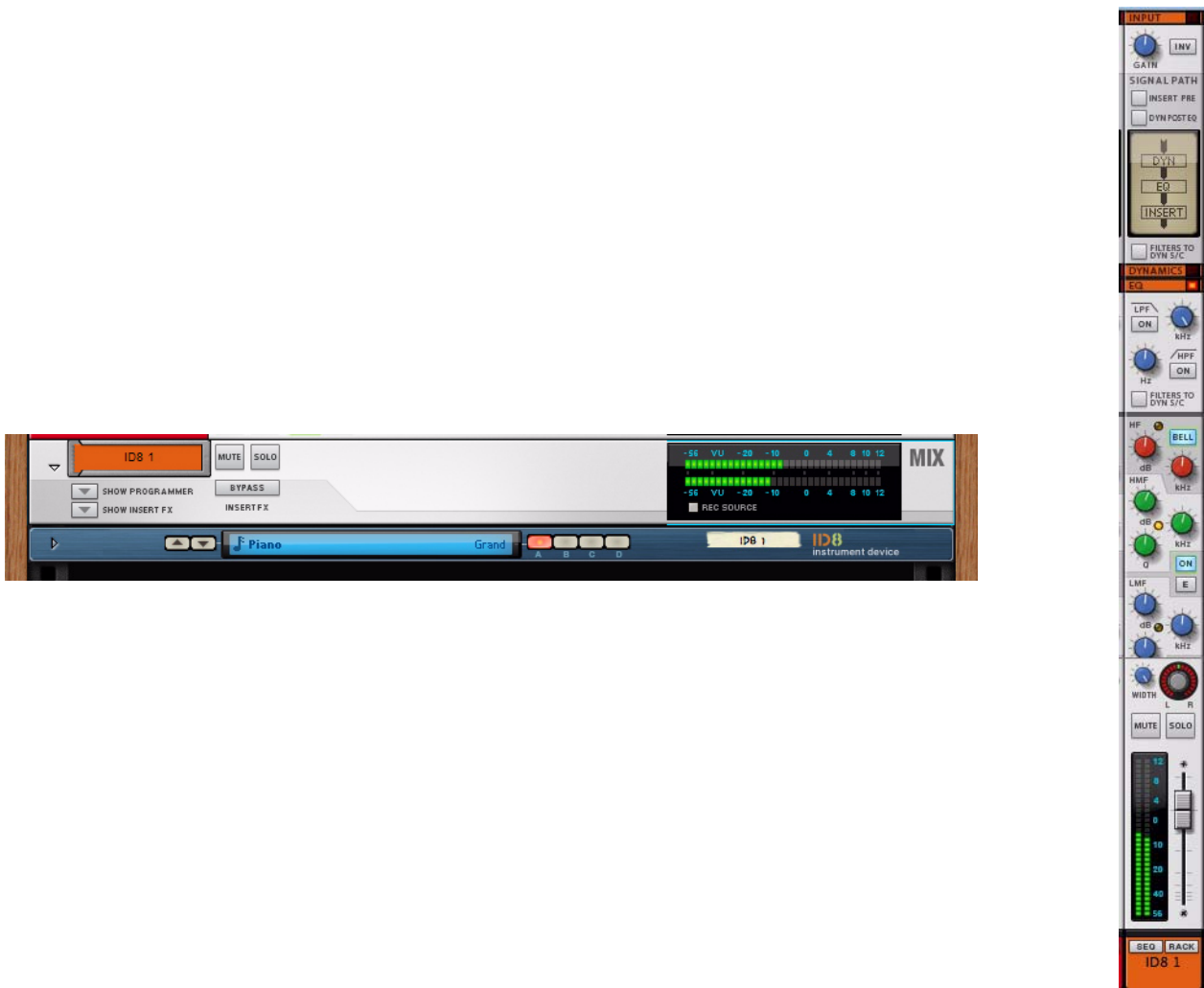
A Mix Channel device (with an ID8 source device connected) and the corresponding channel strip in the Main Mixer.
