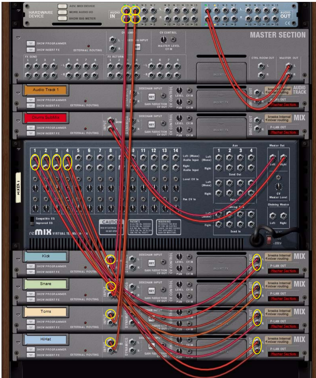
Direct routing of individual Audio Inputs to Mix Channels with their Direct Outs routed for sub-mixing
