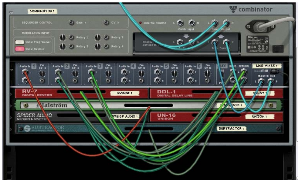
Instrument devices and effects connected to a Line Mixer 6:2 within the Combi.
