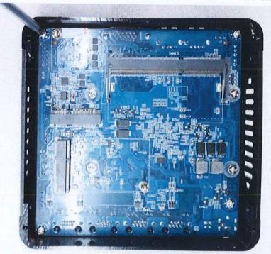
Place screws into the hold to secure the bottom panel to the chassis .
