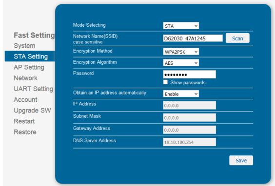
Existing wireless network can be found by clicking the "Scan" button on this page then accessed by configuring the network parameters correctly.
