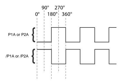
• In quadrature mode, "Pulse output 1" and "Pulse output 2" run at the same pulse rate (set as the "Pulse 1 rate") with a 90° phase shift between the two outputs:
