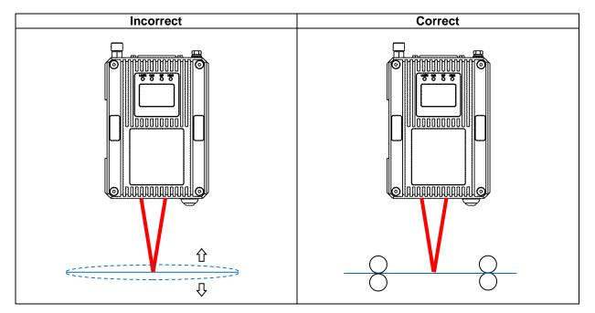
The end-user must provide suitable mechanisms for guiding and stabilising the motion of the measured object.
