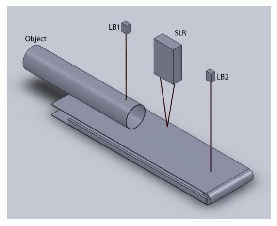
Use two accurately spaced light barriers connected to the logic inputs of the gauge to trigger length measurement only after the object is in position for accurate speed measurement by the gauge.
