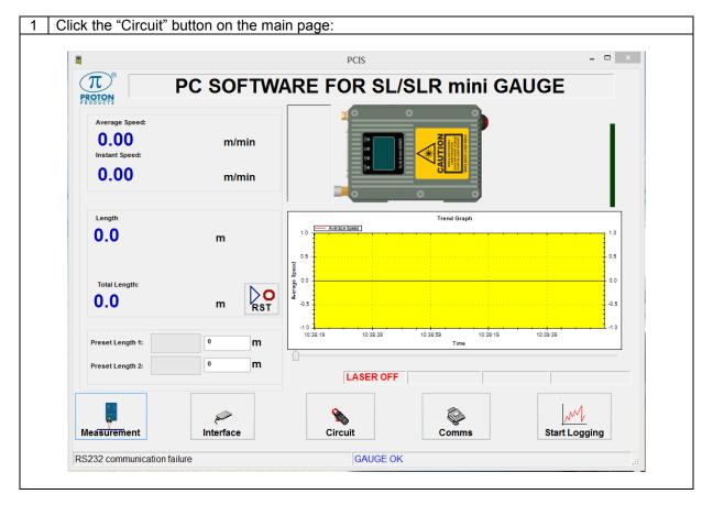
The "Circuit" page displays parameters which may be useful during gauge alignment or for Proton Products authorized service personnel; when contacting Proton Products for technical assistance, please have the information displayed on the "Circuit" page available for our service personnel to better diagnose any problems.
