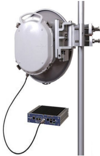
Figure 7: IDU - ODU Cabling
