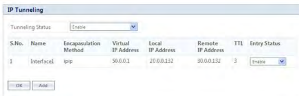
Figure 5-91 IP Tunneling Interfaces
