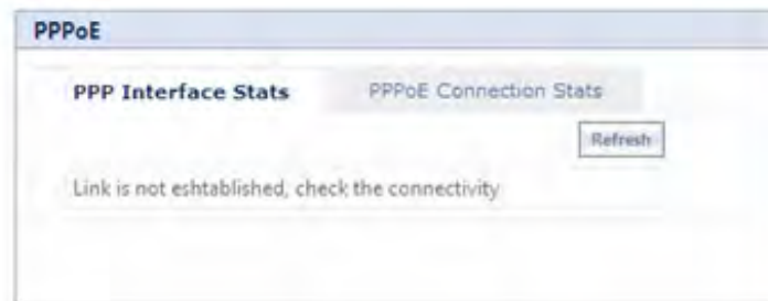
Figure 7-4 PPPoE Server - No Link Established
