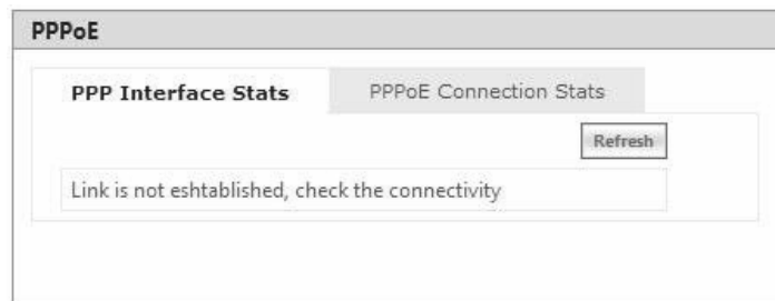
Figure 7-5 PPPoE Server - No Link Established
