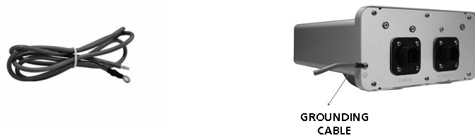
Figure 3-32 Grounding the Device
