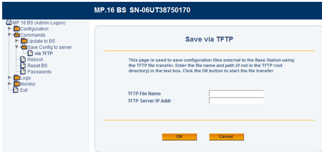
Figure 5-2 Save via TFTP Screen
