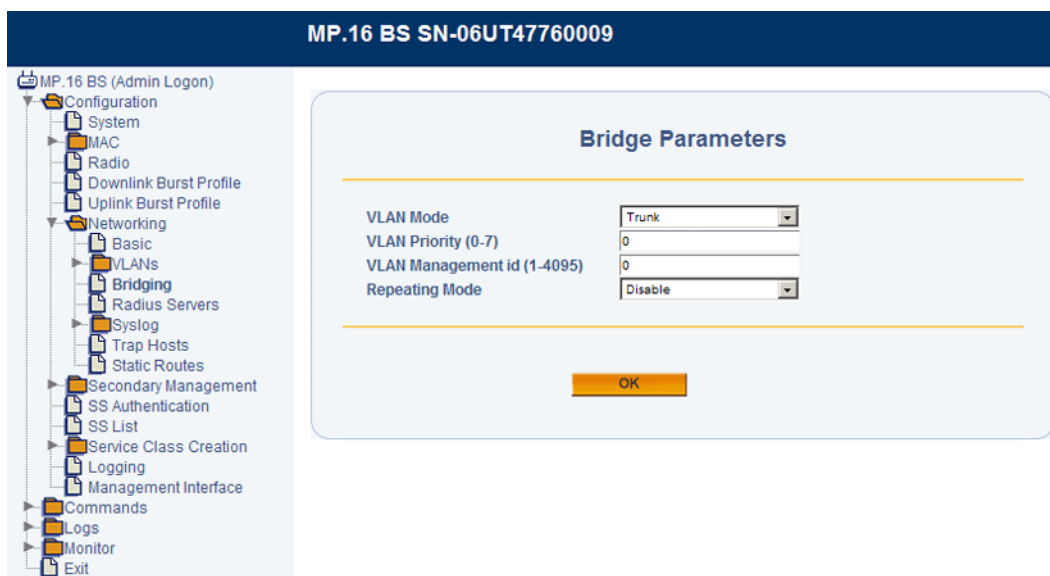
Figure 3-12 Bridge Parameters (Trunk Mode)
