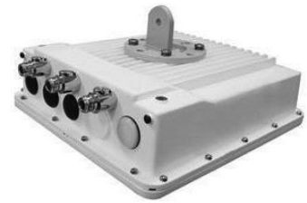
Mounting Plate fixed to the Device
