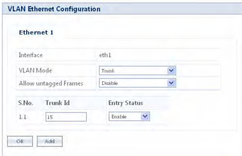
Figure 4-44 VLAN operation in Trunk Mode
