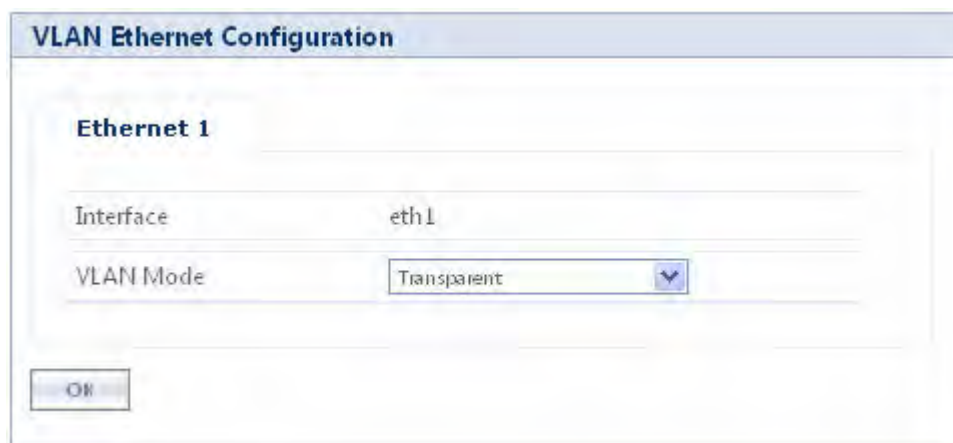
Figure 4-43 VLAN Operation in Transparent Mode
