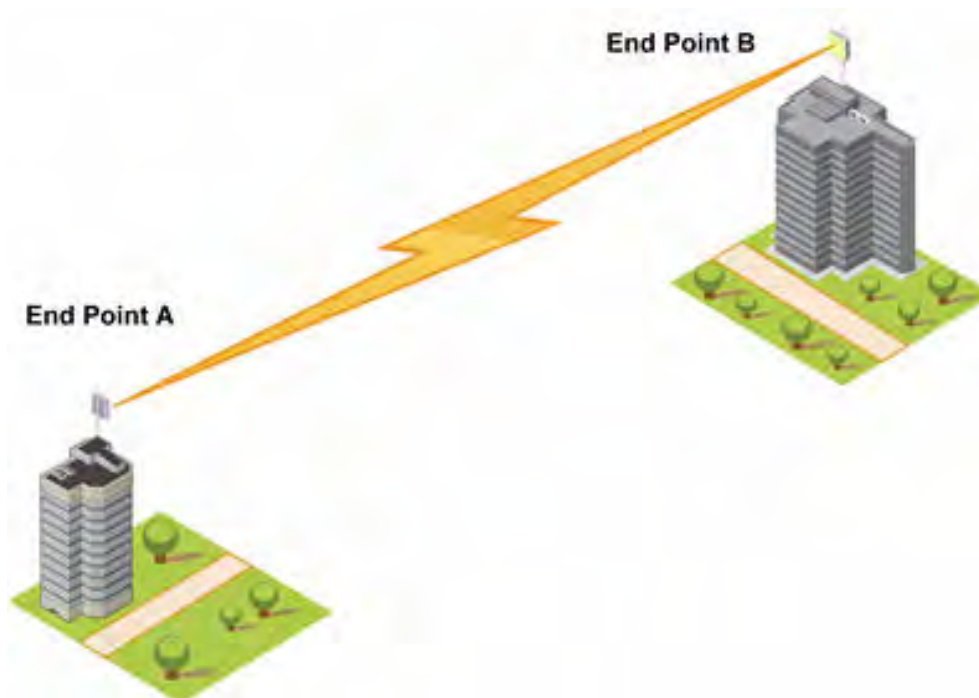
Figure 1-1 Wireless Network Topology (Point-to-Point-Link)
