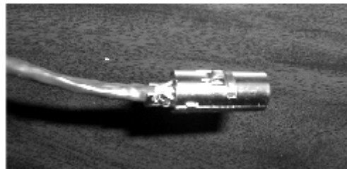
Figure 32. Metal Shell Placed Over 8-Pin DIN Connector
