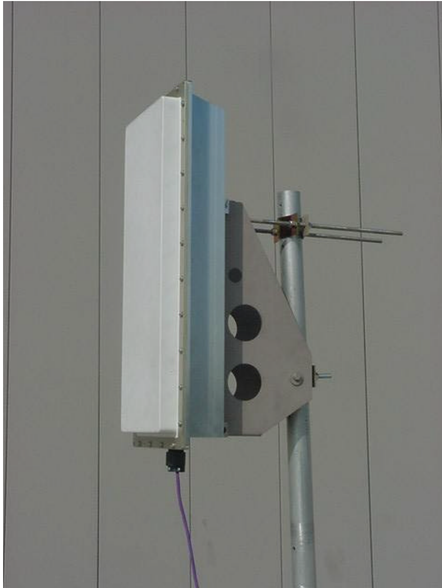
Figure 3-3: Base Station ODU
