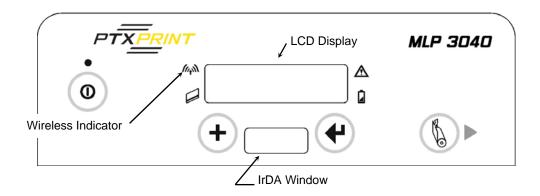
Figure 12 - Wireless Indicator & IrDA Window
