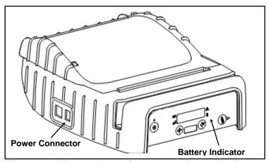
Figure 8 - MLP 3040 Power Connector & Battery Indicator
