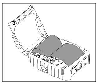
Figure 4 - Paper Laying Through Print Head
