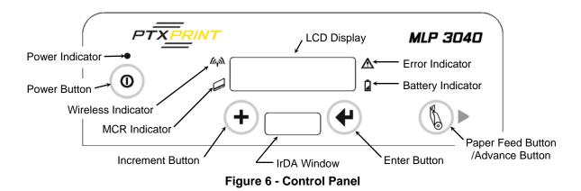
In normal daily use, most users will only use the **O** Power Button/Indicator and perhaps the **Paper Feed** Button, and observe any messages that may appear on the LCD Display. The purpose and functionality of all of the buttons and indicators are listed below.
