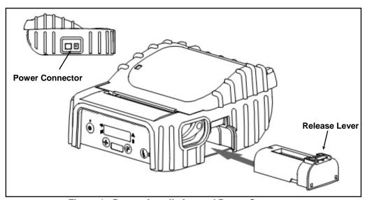
Figure 1 - Battery Installation and Power Connector
