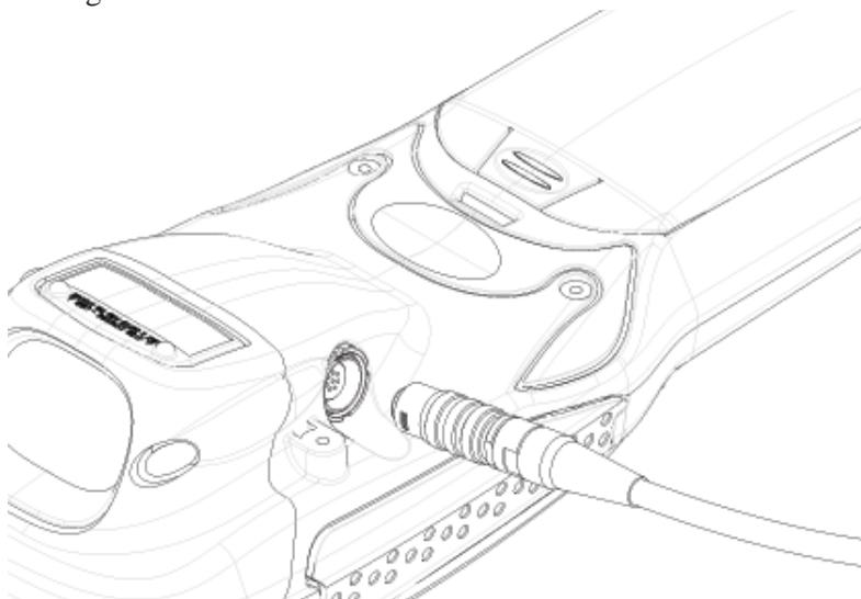
Figure 3.8 Attaching The Cable To The Tether Port
