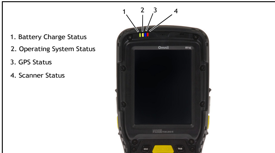
Figure 3.3 LED Status Indicators
