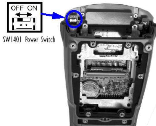
With the power shut down, you can install the RFID Module HF-T2-A1.
