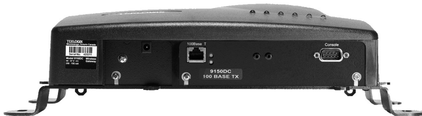
Figure 1.3 The 9150DC Wireless Gateway - Bottom View
