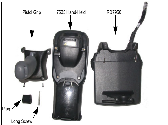
Figure 3.1 RD7950 Installation Components
