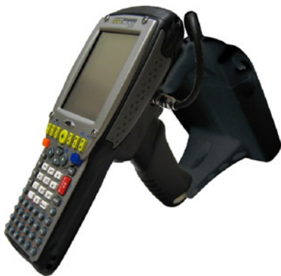
Figure 3.6 RD7950 Installed On 7535 Hand-Held Computer
