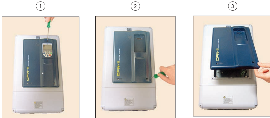
Figure 3.6 - HMI and control rack cover removal
