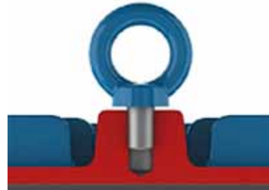
Figure 4.2 - Incorrect tightening of the eyebolt
