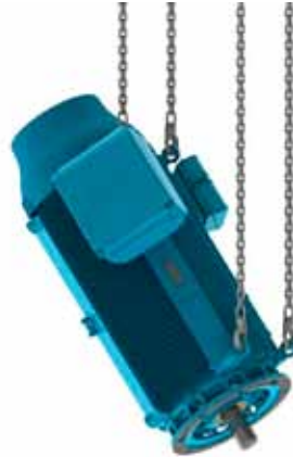
Figure 4.13 - Placing HGF motor in vertical position
