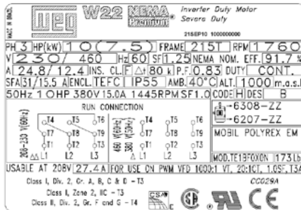
Figure 2.1 - IEC motor nameplate
