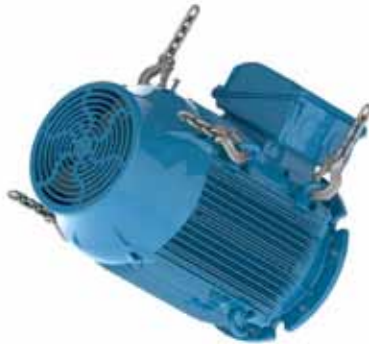
Figure 4.18 - Motor is being rotated to horizontal position
