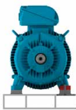
Figure 6.3 - Motor installed on metallic base
