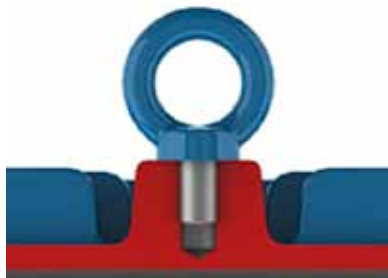
Figure 4.1 - Correct tightening of the eyebolt
