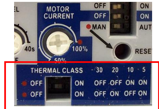
Figure 7 – Thermal Class Dip Switch Location
