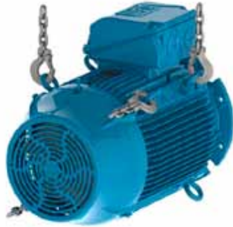
Figure 4.10 - Installation of the second pair of eyebolts
