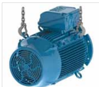
Figure 4.9 - Removing the motor from the packaging
