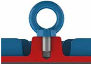
Figure 4.1 - Correct tightening of the eyebolt
