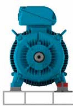
Figure 6.3 - Motor installed on metallic base
