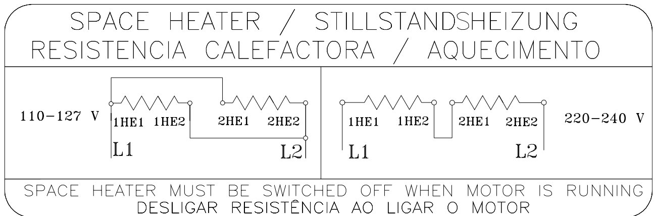
Figure 6.17 - Dual voltage space heater connection
