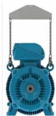
Figure 4.6 - Use of a spreader bar for lifting
