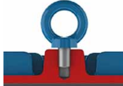
Figure 4.2 - Incorrect tightening of the eyebolt
