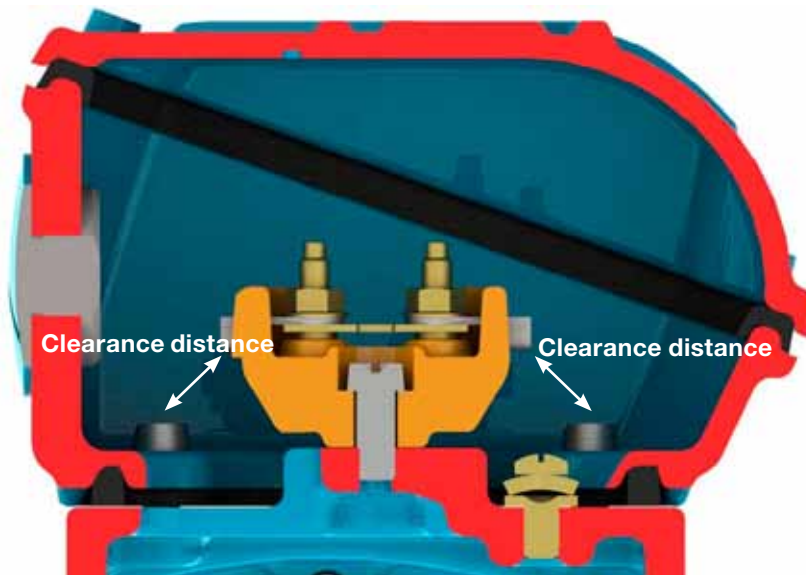
Figure 6.13 - Clearance distance representation
