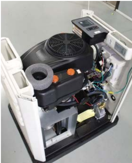
Figure 1.3 — Remove Side Panels
