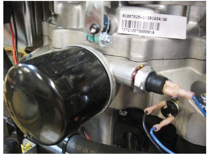
Figure 3.4 – Low Oil Pressure and High Temperature Switches
