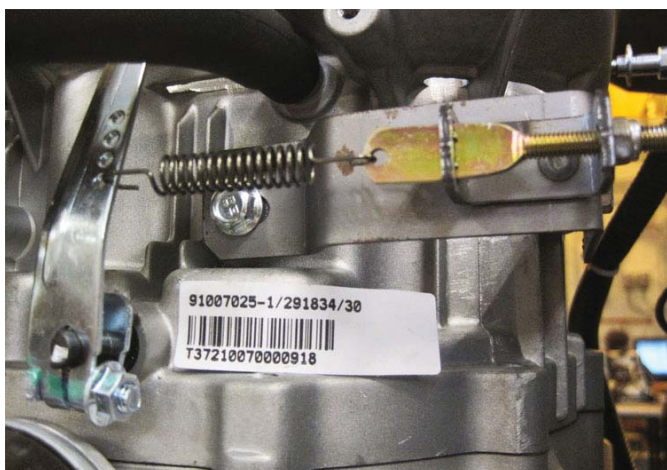
Figure 2.1 — Engine Governor Adjustment Single Cylinder Engines
