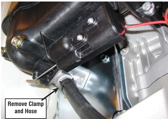
Figure 1.4 — Remove Hose Clamp & Hose
