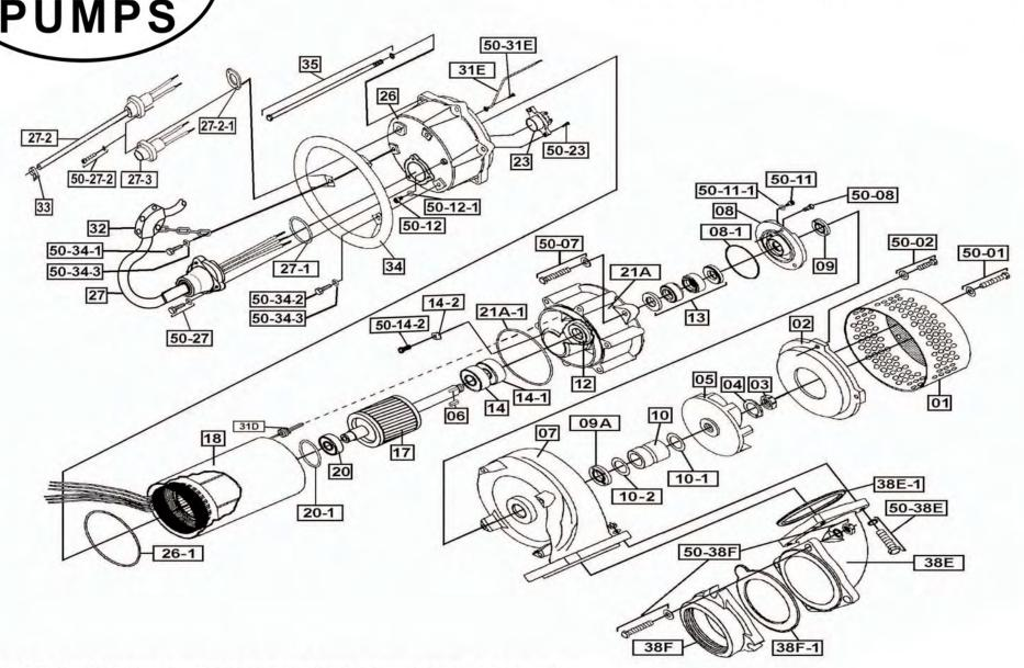
NOTE: Seal Minder (Pos# 27-2, 33, 50-33) is an optional component. JX Series pumps come with Seal Minder cap only (Pos# 27-3)..
