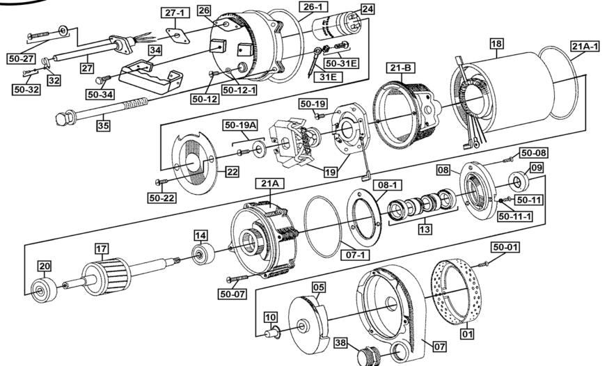
NOTE: Seal Minder (Pos# 27-2, 33, 50-33) is an optional component. JX Series pumps come with Seal Minder cap only (Pos# 27-3)..
