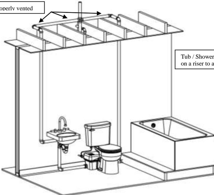
Tub / Shower should be installed on a riser to accommodate the P trap
