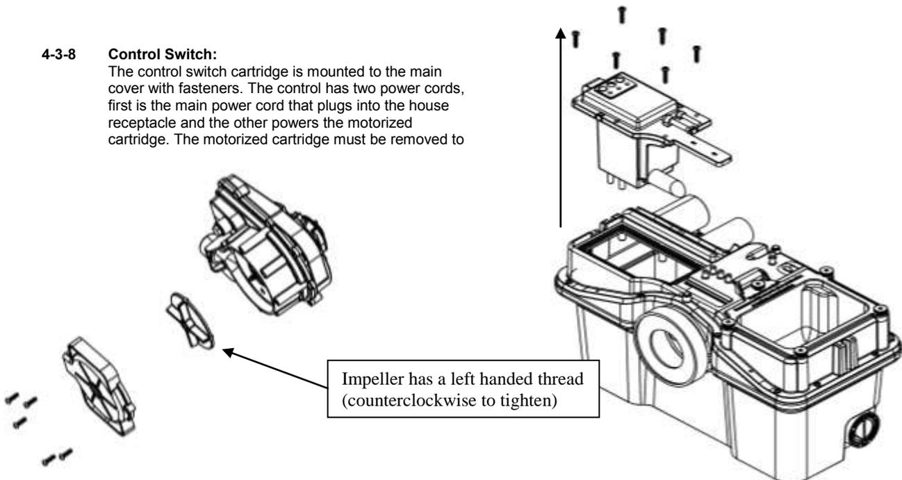
disconnect this cord. See instructions under the heading “Accessibility to Motorized cartridge 4-3-5” for details.
