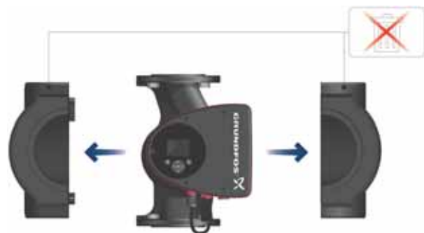
Fig. 3 Fitting insulating shells to the pump
