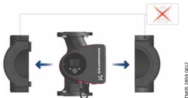
Fig. 3 Fitting insulating shells to the pump
