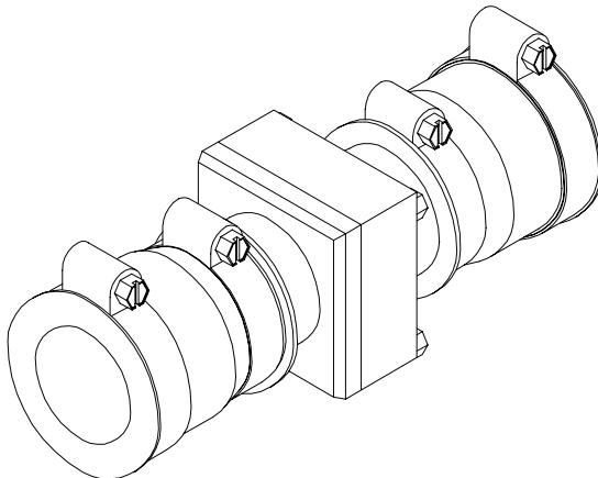
The flapper check valve is used for preventing backflow of materials in waste water lines, sump pump disposal lines, sewage lift stations or ejector systems. Also used where minimum head loss or flow resistance is required, or in swimming pools, hot tubs, or spa applications.
