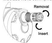
If your installation requires the removal of the in-built check valve or the in-built check valve requires removal for servicing, this can be achieved without difficulty. The in-built check valve is a cassette design, which is screwed in through the suction inlet.
