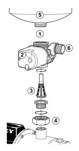
Fit the Supercell pressure tank to the tank connection inlet with thread tape. Firmly hand tighten. Fit the socket to the discharge using thread tape.
