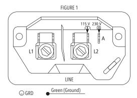
Align black plug to 115 V or 230 V arrow.  $\frac{1}{2}$  HP wired 115 V,  $\frac{3}{4}$  HP and up wired 230 V at factory.
