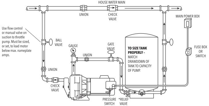
\* NOTE: Required if system pressure can exceed 100 PSI.
