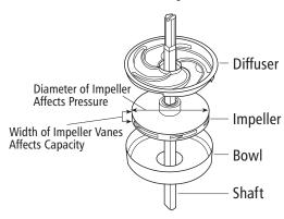
The capacity of a multistage centrifugal pump (submersible) is largely determined by the width of the impeller and diffuser, regardless of the number of stages. The pressure is determined by the diameter of the impeller, the speed at which it rotates and the number of impellers. The diameter is limited to the size of wells drilled. Most submersibles are designed to fit in four or six inch wells (or larger).
