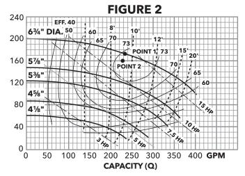
Determine that the new impeller will meet the required capacity:
