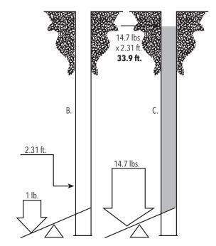
A vacuum gauge indicates total suction lift (vertical lift + friction loss = total lift) in inches of mercury. 1" on the gauge = 1.13 ft. of total suction lift (based on pump located at sea level).
