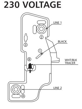
Motor is non-reversible CCW rotation shaft end. Supply connections, use wires sized on the basis of 60°C ampacity and rated minimum 90°C.
