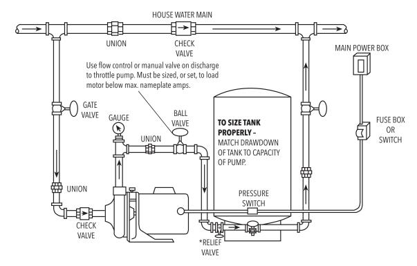
\* NOTE: Required if system pressure can exceed 100 PSI.
