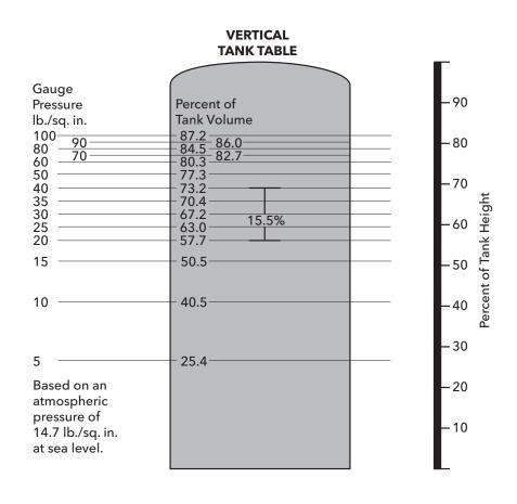
When using large standard galvanized tanks, a constant air cushion is required for proper operation of the water system.
