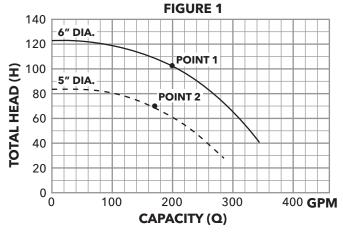
The 5 inch diameter Head/Capacity performance point can be plotted on the graph (figure 1; point 2). By taking additional Head/Capacity points on the 6" diameter curve line and using this procedure, a new Head/Capacity curve line can be produced for the 5 inch diameter impeller.
