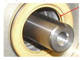
Slide the impeller (9) onto the shaft, being careful not to roll the lips of the mechanical seal (19) backwards.
