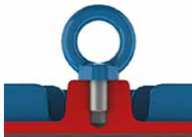
Figure 4.1 - Correct tightening of the eyeboll
