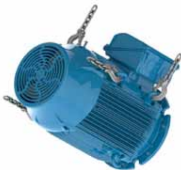
Figure 4.18 - Motor is being rotated to horizontal position
