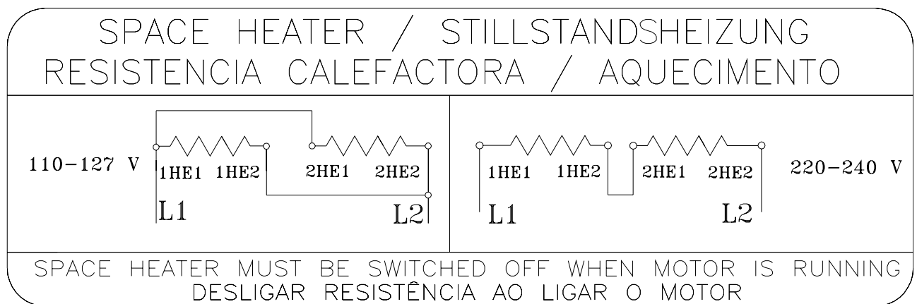
Figure 6.17 - Dual voltage space heater connection
