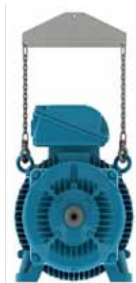
Figure 4.6 - Use of a spreader bar for lifting
