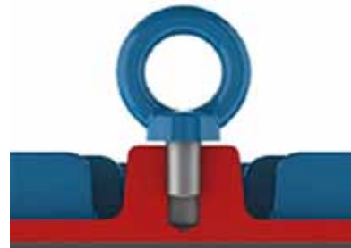
Figure 4.2 - Incorrect tightening of the eyeboll
