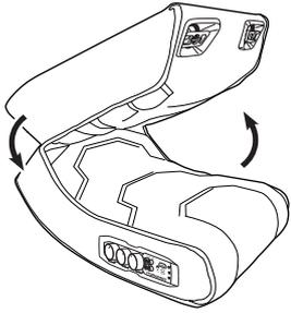
**1** Unfold the top portion of the Sound Rocker until the backrest is flush with the seat portion. Secure velcro tab on the bottom of the rocker.
