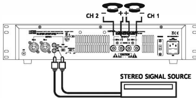
**CAUTION!** Do not use balanced and unbalanced inputs simultaneously!!
