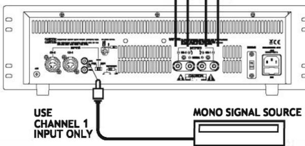
**CAUTION!** Do not use balanced and unbalanced inputs simultaneously!!
