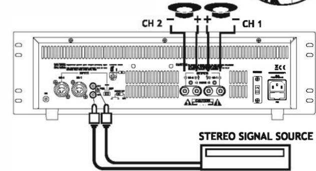
**CAUTION!** Do not use balanced and unbalanced inputs simultaneously!!
