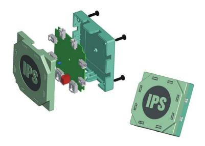
Rigid control module is filled up with non-inflammable potting material to prevent moisture and absorb certain unexpected shock. The module is worked with a video TX transmitter. It may be installed in the boot or lights box. The module could work up to 4 sensors. The module works with different criteria in different heights from 35cm to 80cm.
