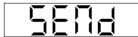
This display shows that Selcall is being sent - ie. in transmit mode.
