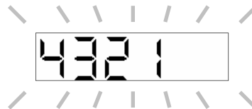
This flashing display shows that you have received a call from Station No. 4321.
