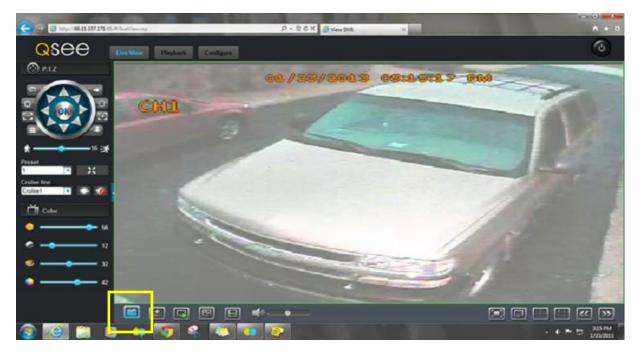
As you can see in the image above the BLUE ICON in the BOTTOM LEFT CORNER of the DVR interface is shaped like a camera. The CAPTURE ICON is what you click on to save the image of your LIVE VIEWING SCREEN onto your remote or local PC. After the Snapshot is taken your PC will display the location were the snapshot is being stored on your PC's hard drive.
