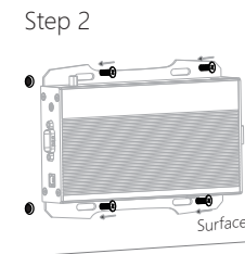
Fix Box PC with screws
