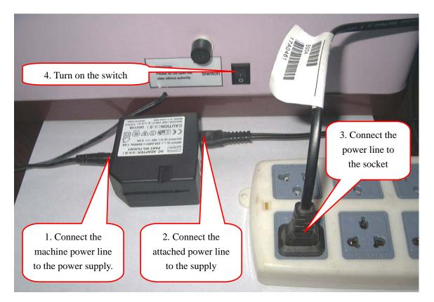
5) The "power light" on the machine will be bright; the "printing status light" inside the machine will be bright also.
