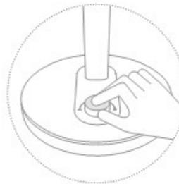
Press and turn the rotating switch to adjust the color temperature
